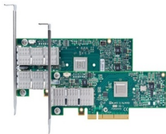
High Performance Interconnects InfiniBand, Omni-Path, EFA <1usec latency, 100Gbps+ Bandwidth
