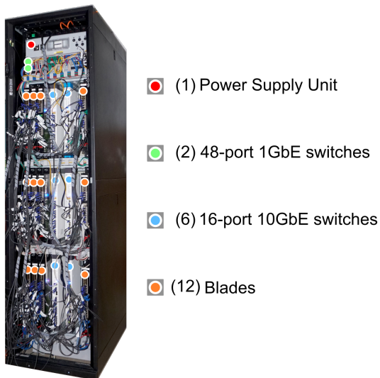
Fig. 8: The ExaNeSt HPC testbed
